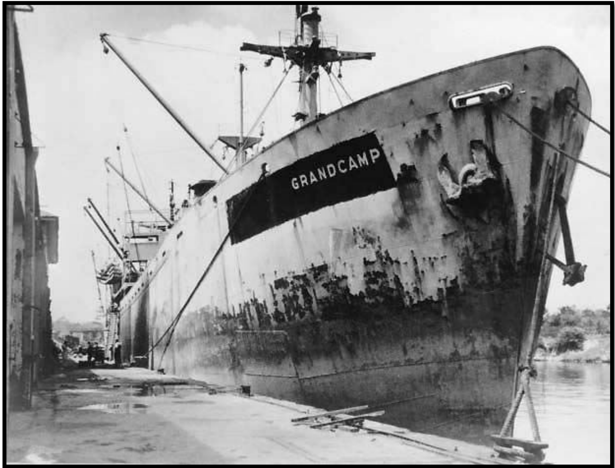
Figure 3: Photograph of the SS Grandcamp prior to the explosion and fire at Texas City, Texas in April of 1947. A combination of fire in the hold of the ship containing ammonium nitrate and steam pumped into the hold of the ship to extinguish the fire caused the largest non-nuclear explosion in United States history. The cause of the fire was never determined.
